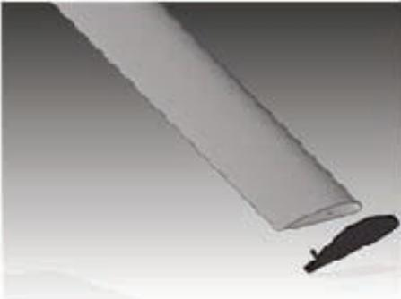
*Loosen the screw fissing the plastic Winglet to the blade*
