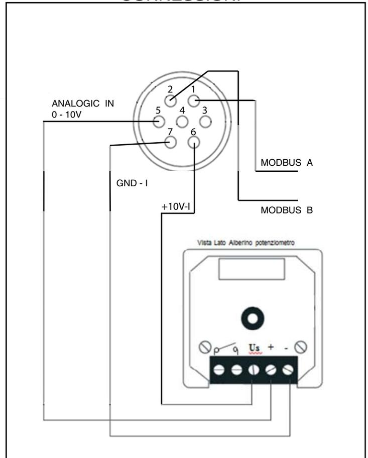
NB: It is necessary pull the A and B wires down to the control box for the Modbus connection, used for maintenance and diagnostic actions.
